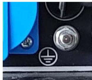
The ground terminal is designed to prevent electric shock by connecting it to the ground wire. The generator must be properly grounded before operation, use a copper wire with a diameter equal to or greater than the one of the power cables of the connected appliance.
